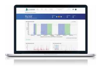
The StormHarvester System system uses weather forecasts and historic network performance to predict future network behaviour. Once a potential flood/overflow event is identified, the system runs thousands of scenarios in real time to determine the optimum operational sequence to minimise or prevent overflows. The system then automatically operates the infrastructure according to this sequencing.
